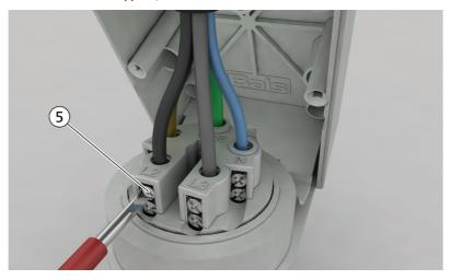
4. Pull out the cable from the housing, and for surface mounting socket outlets and plugs, also out of the cable gland (4).
